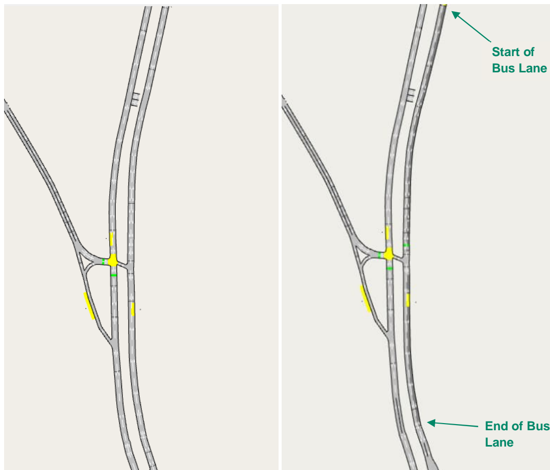
Figure 5 – Otley Road Southbound Without Bus Lane (Left), Otley Road Southbound Including Bus Lane (Right)
