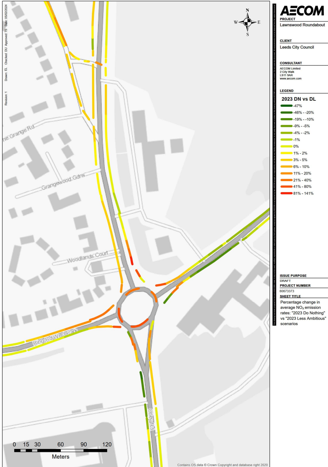
Figure 9 - Percentage change in average NO x emission rates: "2023 Do Nothing" vs "2023 Less Ambitious", Core Tests
